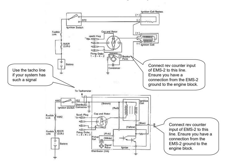
Electronic ignition system with conventional ignition coil
