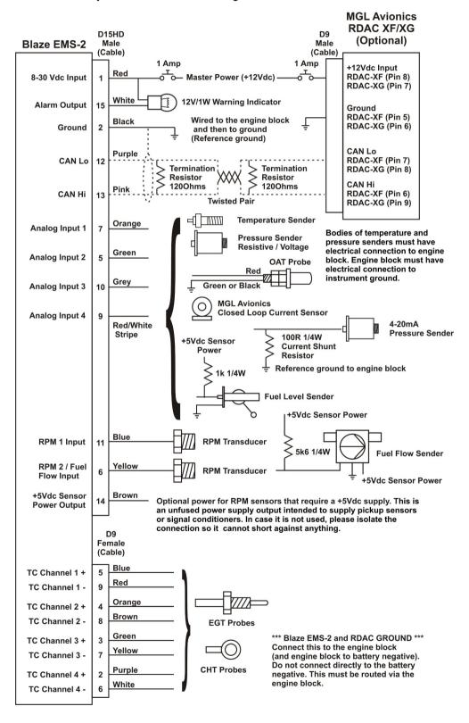
**Please note:** The +5V Sensor power output line is unprotected and intended only for the supply of a hall-effect, optical or gear tooth sensors. Connecting any voltages (such as the 12V supply) to this line could destroy the instrument. The +5V line may supply currents of up to 50mA. Should your sensor require greater currents you must supply it from another source.
