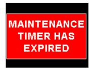
A maximum of 999 hours can be entered as a maintenance interval. A reminder message will appear on startup when zero hours are remaining. The reminder message will disappear after the pilot presses any key. Engine running time for the purpose of the mainteance timer is defined as the run time where the engine RPM is greater than the "HOBBS RPM" value as set in the "TIMERS SETUP".
