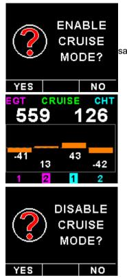
Once in the cruise, press the F2/Down button to enable the Cruise Mode. The "CRUISE" label is displayed at the top of the main display to clearly differentiate it from the normal operating mode. All EGT and CHT readings are immediately sampled as reference temperatures for the cruise.
