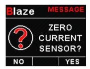
Select this function to indicate to the EMS-2 that zero current is flowing through the MGL Avionics Closed Loop Current sensor. This is best done with the MGL Closed Loop Current sensor disconnected from the main current supplying conductor.
