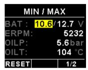
This display can be accessed by rotating the rotary control during the normal display mode. Press the F1/Up button when the max values display is showing to reset the maximum values.
