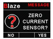
Select this function to indicate to the EMS-2 that zero current is flowing through the MGL Avionics Closed Loop Current sensor. This is best done with the MGL Closed Loop Current sensor disconnected from the main current supplying conductor.
