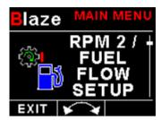
The RPM-2 input can be used for RPM or fuel flow.
