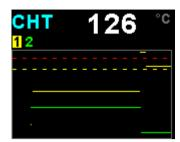
This display can be accessed by rotating the rotary control during the normal display mode. The trend graph displays the last 160 seconds of EGT/CHT temperature readings.
