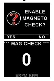
Press the F2/Down button once you have reached your normal run-up RPM. The display will show the RPM deviation from when the magneto function was activated. Any RPM drops will be displayed as a negative RPM value, a positive reading indicates an increase in RPM.
