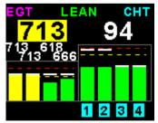
Fuel mixture should be adjusted once you have decided on a suitable cruise power setting (typically 70%). Press the F1/Up button on the main display to enable the engine leaning mode. The "LEAN" label is displayed at the top of the main display to clearly differentiate it from the normal operating mode.
