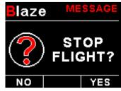
Press the F1/Up button during the normal display mode to manually start/stop a flight. This key is only active if the EMS-2 is setup to select the manual flight option under the "TIMERS" setup menu.
