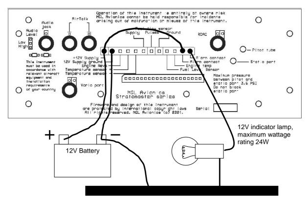
Please note: The drawing above leaves out the switch between the (+) terminal of the battery and the *Stratomaster E2* unit for the sake of clarity.
