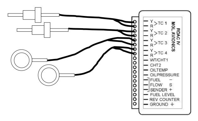
The thermocouple amplifier is a precision device providing full cold junction compensation and bow voltage correction. In addition the amplifier measures and corrects for its own errors. This results in very accurate measurements providing you install high quality probes. Here are some guidelines:
