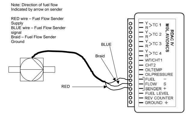
Warning: Incorrect wiring can damage both the RDAC unit as well as the flow sender.
