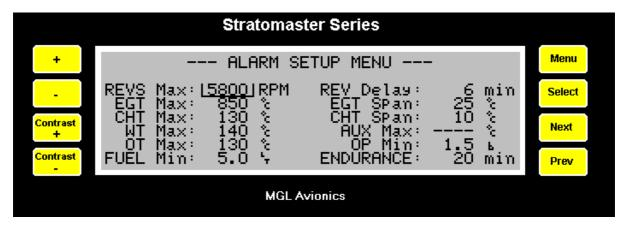
The engine *Revs Delay* option allows a delay to be set with the alarm only triggering after the over-rev condition has continued for this period. This allows use with engines such as the Rotax 914 with turbo-charger where over-revs are only considered a problem once they have been continued for six minutes or more. If the over-rev condition, exceeds the *Max Revs* value specified under the *Range Menu*, the delay is ignored and the alarm triggers instantly.
