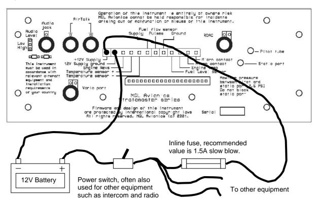
Generally it is not required to fit any form of power supply filters or surge suppressers as the *Stratomaster E2* includes the required protection devices. External power line filters or surge protectors should only be considered in very unusual conditions.
