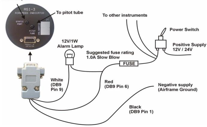
The use of an external 1A fuse is recommended. Connect the supply terminals to your aircrafts power supply. The ASI-3 can be used on both 12V and 24V without the use of any pre-regulators. Ensure that the supply voltage will not drop below 8V during operation as this may result in incorrect voltage and or current readings.
