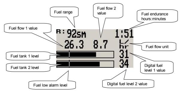
3.3 Single fuel flow and dual fuel level senders (dual tank) Differential fuel flow and dual fuel level senders (dual tank) Summed fuel flow and dual fuel level senders (dual tank)
